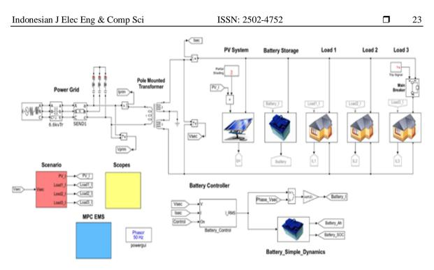
Figure 2. Simulink microgrid model
