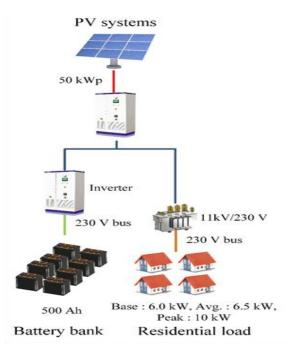
Figure 1. Microgrid schematic
