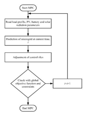
Figure 3. MPC control scheme
