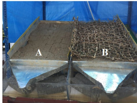
Figure 1. Experimental soil testbeds with slope of 30 degree setup for A) bare soil; and B) WHFM
