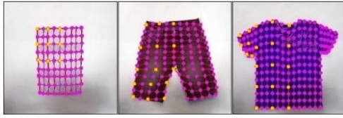
Figure 10. Annotation points for hanging the spread-out garment mesh model before image acquisition.
