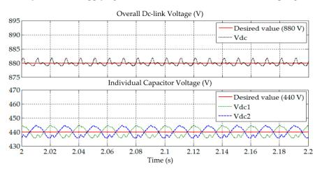
**Figure 16.** Simulation result obtained under Scenario II for Load B, showing the overall dc-link voltage  $V_{dc}$ , and individual voltage of each split capacitor  $V_{dc1}$  and  $V_{dc2}$ , demonstrated by SAPF while applying the enhanced-ADALINE algorithm.
