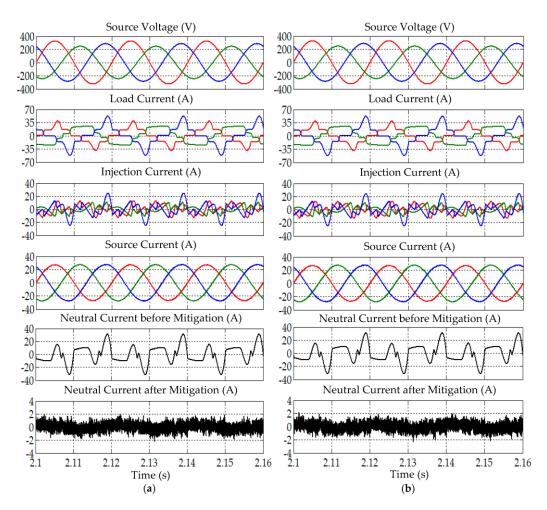
**Figure 13.** Simulation results obtained under Scenario II for Load A, showing source voltage  $v_{Sabc}$ , load current  $i_{Labc}$ , injection current  $i_{injabc}$ , source current  $i_{Sabc}$ , and neutral current before and after mitigation, demonstrated by SAPF while applying the (**a**) enhanced-ADALINE and (**b**) STF-dq0 algorithms.
