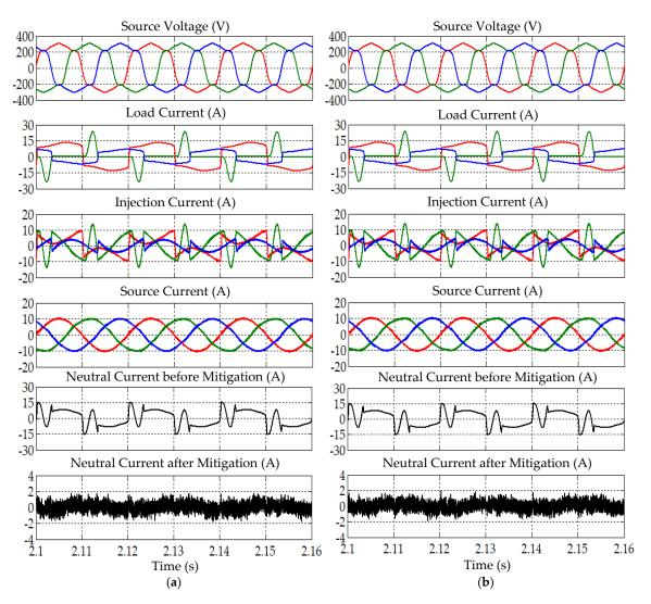
**Figure 10.** Simulation results obtained under Scenario I for Load B, showing source voltage  $v_{Sabc}$ , load current  $i_{Labc}$ , injection current  $i_{injabc}$ , source current  $i_{Sabc}$ , and neutral current before and after mitigation, demonstrated by SAPF while applying the (**a**) enhanced-ADALINE and (**b**) STF-dq0 algorithms.
