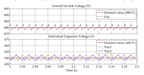
**Figure 11.** Simulation result obtained under Scenario I for Load B, showing the overall dc-link voltage  $V_{dc}$ , and individual voltage of each split capacitor  $V_{dc1}$  and  $V_{dc2}$ , demonstrated by SAPF while applying the enhanced-ADALINE algorithm.
