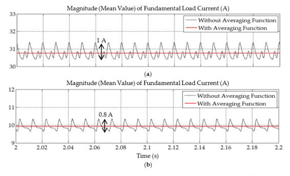
**Figure 7.** Simulation result obtained under Scenario I, showing the magnitude (mean value) of fundamental load current extracted by the enhanced-ADALINE algorithm with and without integrating Averaging function: (a) Load A and (b) Load B.
