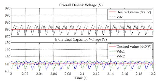
**Figure 14.** Simulation result obtained under Scenario II for Load A, showing the overall dc-link voltage  $V_{dc}$ , and individual voltage of each split capacitor  $V_{dc1}$  and  $V_{dc2}$ , demonstrated by SAPF while applying the enhanced-ADALINE algorithm.
