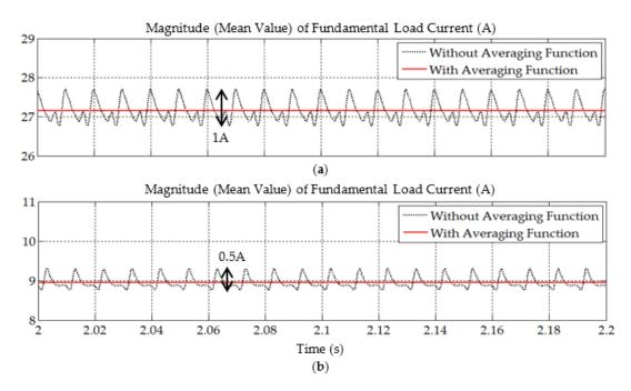
**Figure 17.** Simulation result obtained under Scenario III, showing the magnitude (mean value) of fundamental load current extracted by the enhanced-ADALINE algorithm with and without integrating Averaging function: (**a**) Load A and (**b**) Load B.
