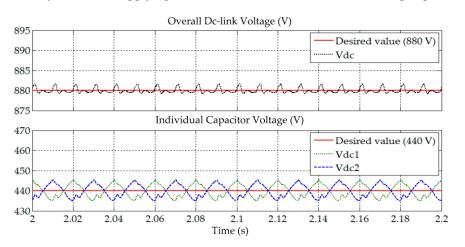
**Figure 21.** Simulation result obtained under Scenario III for Load B, showing the overall dc-link voltage  $V_{dc}$ , and individual voltage of each split capacitor  $V_{dc1}$  and  $V_{dc2}$ , demonstrated by SAPF while applying the enhanced-ADALINE algorithm.
