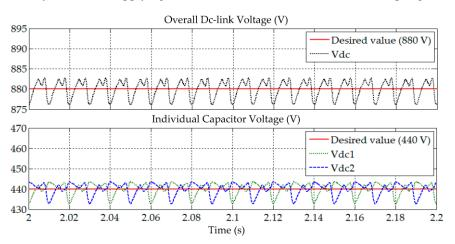
**Figure 19.** Simulation result obtained under Scenario III for Load A, showing the overall dc-link voltage  $V_{dc}$ , and individual voltage of each split capacitor  $V_{dc1}$  and  $V_{dc2}$ , demonstrated by SAPF while applying the enhanced-ADALINE algorithm.
