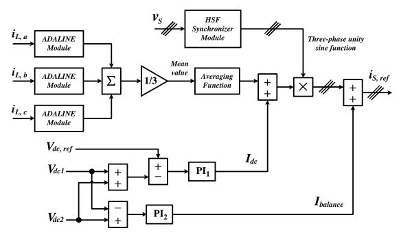
Figure 4. Control structure of the enhanced-ADALINE algorithm.
