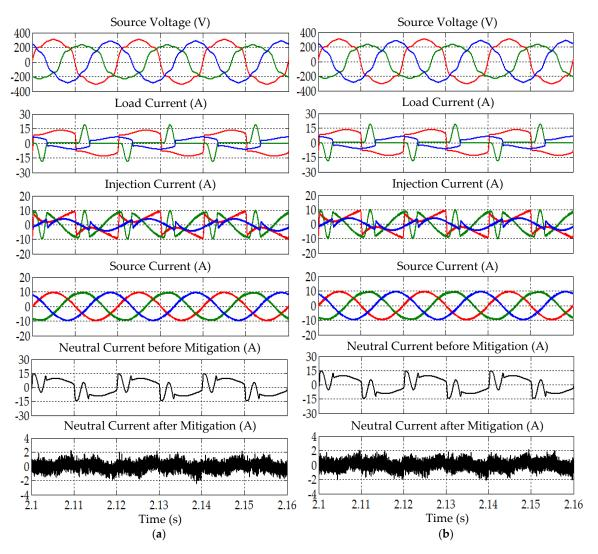
**Figure 20.** Simulation results obtained under Scenario III for Load B, showing source voltage  $v_{Sabc}$ , load current  $i_{Labc}$ , injection current  $i_{injabc}$ , source current  $i_{Sabc}$ , and neutral current before and after mitigation, demonstrated by SAPF while applying the (**a**) enhanced-ADALINE and (**b**) STF-dq0 algorithms.
