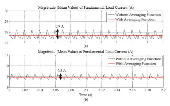
**Figure 12.** Simulation result obtained under Scenario II, showing the magnitude (mean value) of fundamental load current extracted by the enhanced-ADALINE algorithm with and without integrating Averaging function: (**a**) Load A and (**b**) Load B.
