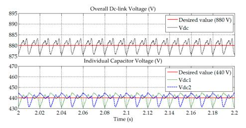
**Figure 9.** Simulation result obtained under Scenario I for Load A, showing the overall dc-link voltage  $V_{dc}$ , and individual voltage of each split capacitor  $V_{dc1}$  and  $V_{dc2}$ , demonstrated by SAPF while applying the enhanced-ADALINE algorithm.
