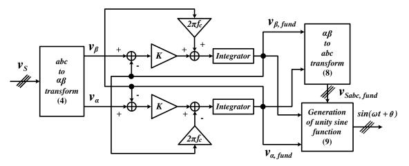
Figure 3. Control structure of a highly selective filter (HSF) synchronizer module.
