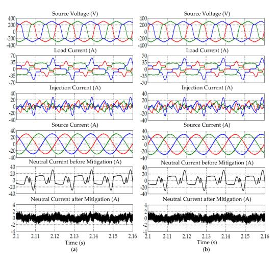
**Figure 8.** Simulation results obtained under Scenario I for Load A, showing source voltage  $v_{Sabc}$ , load current  $i_{Labc}$ , injection current  $i_{injabc}$ , source current  $i_{Sabc}$ , and neutral current before and after mitigation, demonstrated by SAPF while applying the (**a**) enhanced-ADALINE and (**b**) STF-dq0 algorithms.
