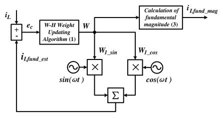
Figure 2. Control structure of a generalized adaptive linear neuron (ADALINE) module [11,19].
