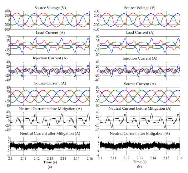
**Figure 18.** Simulation results obtained under Scenario III for Load A, showing source voltage  $v_{Sabc}$ , load current  $i_{Labc}$ , injection current  $i_{injabc}$ , source current  $i_{Sabc}$ , and neutral current before and after mitigation, demonstrated by SAPF while applying the (**a**) enhanced-ADALINE and (**b**) STF-dq0 algorithms.
