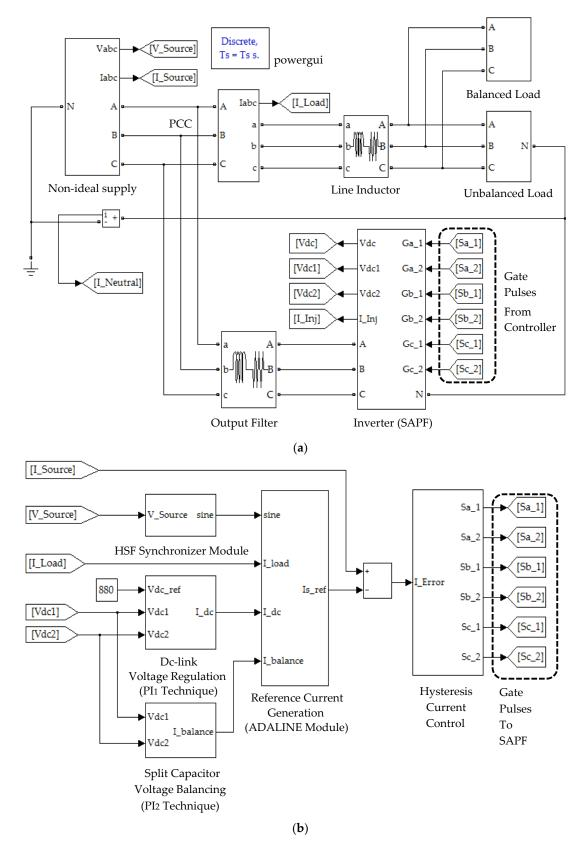
**Figure 5.** Simulation model of SAPF in a three-phase four-wire system: (**a**) connection of power circuits, and (**b**) control algorithms that constituted the control system.
