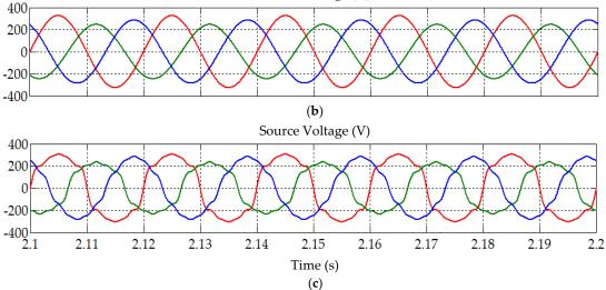
**Figure 6.** Non-ideal source voltages considered in this work: (**a**) balanced and distorted (Scenario I), (**b**) unbalanced and sinusoidal (Scenario II), and (**c**) unbalanced and distorted (Scenario III).
