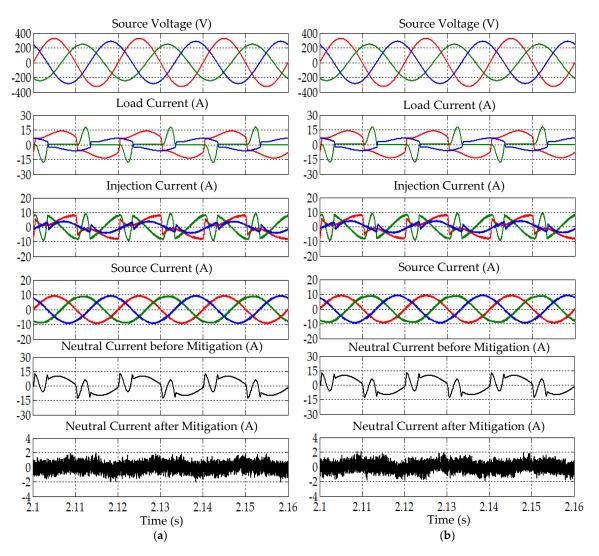
**Figure 15.** Simulation results obtained under Scenario II for Load B, showing source voltage  $v_{Sabc}$ , load current  $i_{Labc}$ , injection current  $i_{injabc}$ , source current  $i_{Sabc}$ , and neutral current before and after mitigation, demonstrated by SAPF while applying the (**a**) enhanced-ADALINE and (**b**) STF-dq0 algorithms.
