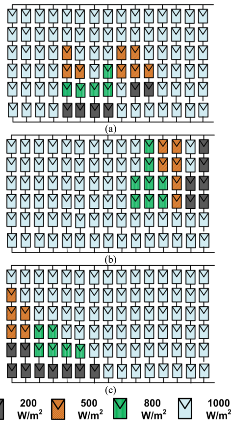
Fig. 4. Photovoltaic Array under Partial Shading Condition, (a) Case 1, (b) Case 2 (c) Case 3.
