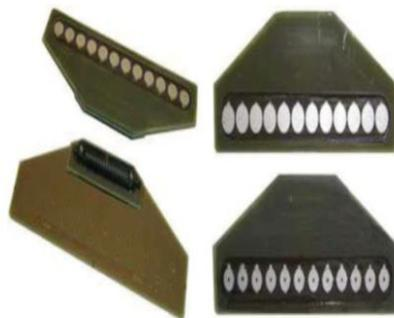
Figure 2.19 Design of SHM Piezoelectric module
