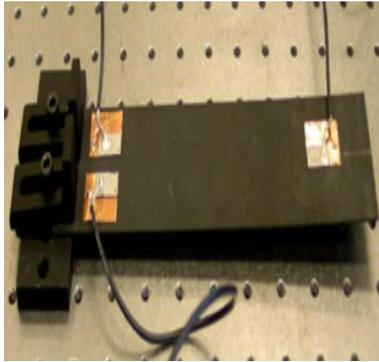
Figure 2.22 Piezoelectric for guide wave design
