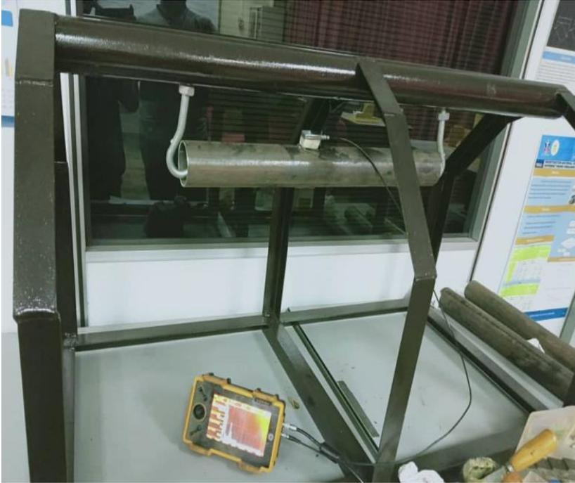
Figure B1.7 Ultrasonic Probe Measuring Pipe Defect
