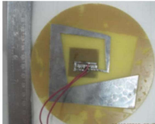
Figure 2.25. Broadband bent triangular monopole presented in [77].
