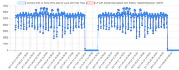
Figure 11. Typical monthly load profile for a commercial customer after BESS installation
