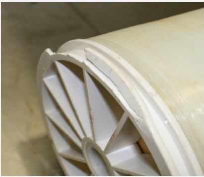
2(d) Improper seal installation
