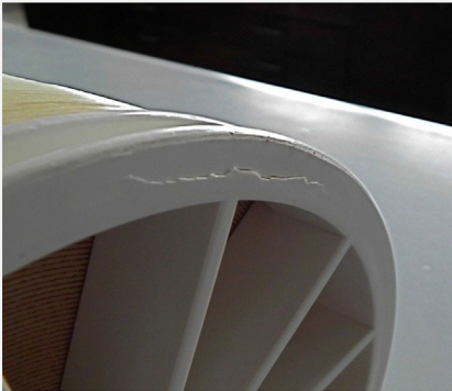
2(b) Cracks in module end caps
