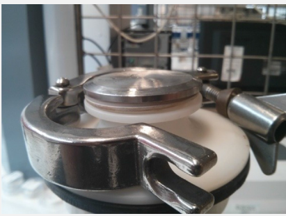
2(d) Improper seal installation
