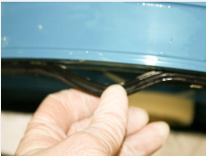
2(c) Module seal failure
